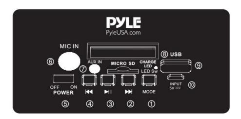
1. Short press to choose input signal, press and hold to turn off front light
