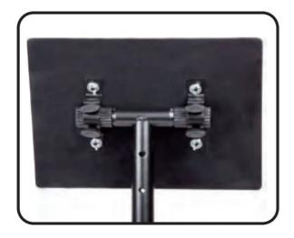
The plate bolts are to be inserted from the top of the unit, going downward through the device resting plate, and out of the other end to meet the metal mounting brackets. The metal mounting bracket clamps can be adjusted or loosened accordingly to allow for angle/tilt adjustment.
