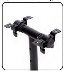
Use the included hardware to secure the device resting plate with the metal mounting clamps. The holes in the mounting clamp brackets should align with the holes protruding through the base plate. Be sure to use a washer between the wing nut and the metal mounting clamp when securing.
