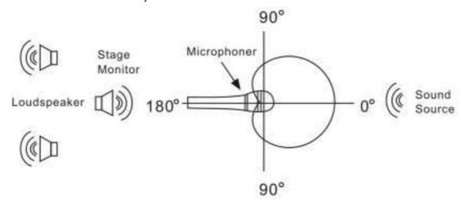
2. Do not cover any part of the grille with your hand, covering the grille alters the sound and distorts the polar pattern in creasing the chance for feedback.
