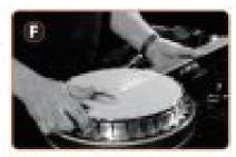
Replace the resonator to the banjo assembly and tighten back all the thumb screws.
