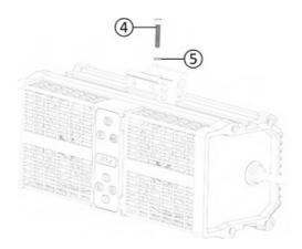
2. Align the screw holes at the bottom of the clamps with the positioning holes that have been made in the slider and lock the M5X24mm screws and M5 spring washers to fix the clamps.
