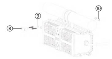
5. Use M6X60mm screws and M6 spring washers to pass through the aluminum ring and the base and the M6 non-slip nut at the back to fix the aluminum ring on the base as shown in the figure. Each nut should be installed in the hexagonal groove.
