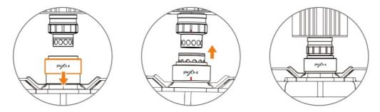
**Note:** After installation, firmly pull the steering wheel backward to confirm secure attachment. If loose, rotate the steering wheel slightly or reinstall it and repeat the check.
