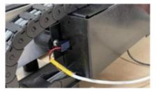
This is a Molex connector and the control cable we include in your kit will have this on the end, so it'll be easy to plug into.
