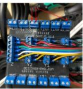
You'll be attaching the PWM cable's RED wire into the "PWM" and BLACK into the "GND" pins found along the left side of the Demon controller's terminal board.
