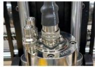
The other end of the spindle cable will plug into the side of our VFD enclosure completing the motor installation.
