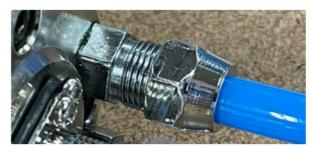
There are two tube connection points and they both will act as either an inlet or outlet depending on how your pump is attached. There is no advantage one way or the other when hooking these up. Unthread the tube nuts and dispose of the black filler piece if it's present. Slide the nut over the tube and press the tube onto the nipple of the connector still attached to the top of your spindle motor. Then thread the nut down over the nipple to securely hold the tube in place.
