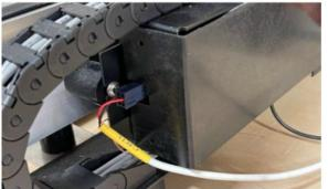
This is a Molex connector and the control cable we include in your kit will have this on the end, so it'll be easy to plug into. Note that the Molex connector is brand new and will likely be hard to plug in. Consider removing your controllers cover so you can grab the backside of the connector soldered to the controller for additional leverage.
