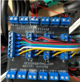
You'll be attaching the PWM cable's RED wire into the "PWM" and BLACK into the "GND" pins found along the left side of the Demon controller's terminal board.
