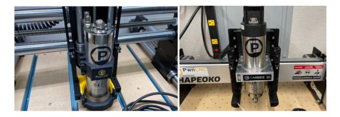
Note: If you're replacing a Dewalt with its' 69mm mount with any of our spindles... you will need a different router mount, or a mount "insert" which converts the 69mm mount to a 65mm mount. Additionally, if you're installing one of our 80mm spindles, you'll need a whole new router mount which is most often purchasable from the maker of your CNC machine.
