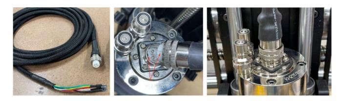
Once you've aligned the cable with the notch, press the connector onto the motor and twist the metal threading nut into place. There is no need to overtighten this nut, a simple hand tightness is sufficient.
