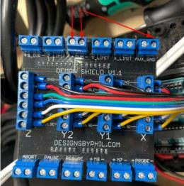
You'll be attaching the PWM cable up to the "PWM" and "GND" pins found along the left side of the Demon controller's terminal board.
