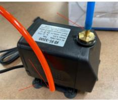
Your kit will come with two coolant tubes, and a pond-pump. I've added enough tubing to run both tubes through a cable chain if it's large enough to support the tubes.
