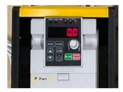
Ensure the Manual Override switch on the left side of the VFD/Enclosure is switched to "1" or up. This will let you use your spindle in manual mode which is very similar to how you used your palm router previously. We'll discuss automatic mode later in this manual.
