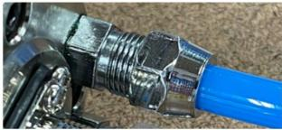
There are two tube connection points and they both will act as either an inlet or outlet depending on how your pump is attached. There is no advantage one way or the other when hooking these up.
