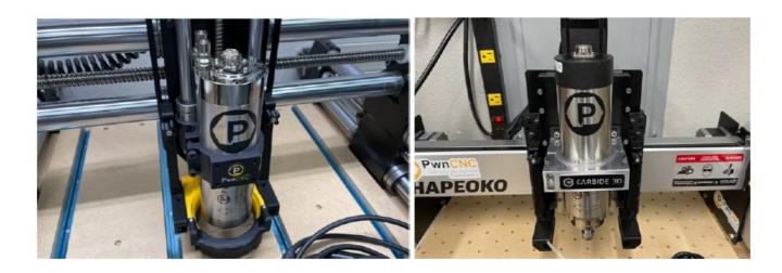
**Note:** If you're replacing a Dewalt with its' 69mm mount with any of our spindles... you will need a different router mount, or a mount "insert" which converts the 69mm mount to a 65mm mount.
