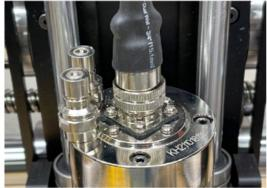
Once you've aligned the cable with the notch, press the connector onto the motor and twist the metal threading nut into place. There is no need to overtighten this nut, a simple hand tightness is sufficient.
