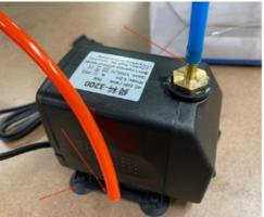
• Your kit will come with two coolant tubes, and a pond-pump. I've added an extra tube so there's enough length to run both tubes through a cable chain if you have one large enough.
