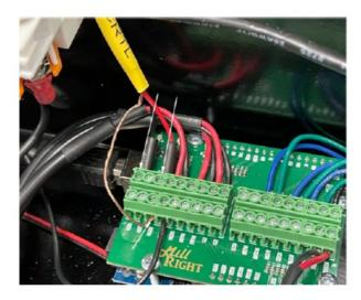
You'll be attaching the PWM cable up to the "PWM" and "GND" pins found along the top-left side of the Mill Right terminal board.
