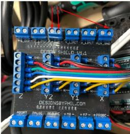
You'll be attaching the PWM cable up to the "PWM" and "GND" pins found along the left side of the Demon controller's terminal board.
