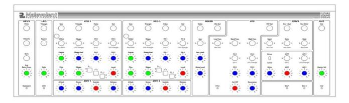
Blue are at minimum or turned fully anti-clockwise Red are at maximum or turned fully clockwise Green are at mid-position or 12 o'clock
