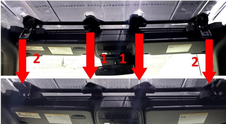
6. Turn the Rear wing clamps starting with the center two clamps
