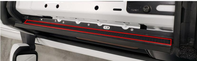
3. Attach the foam seal to the Velcro on the vehicle.
