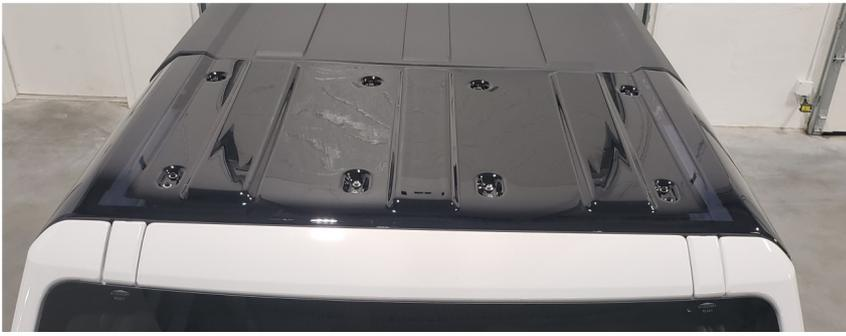
5. Turn the front wing latches then close the two front clamps.
