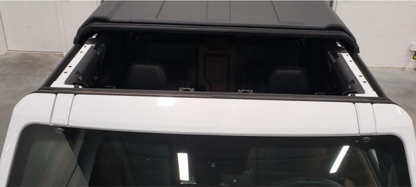
2. Remove the Velcro strip from the foam seal and attach to the vehicle above the door frame.
