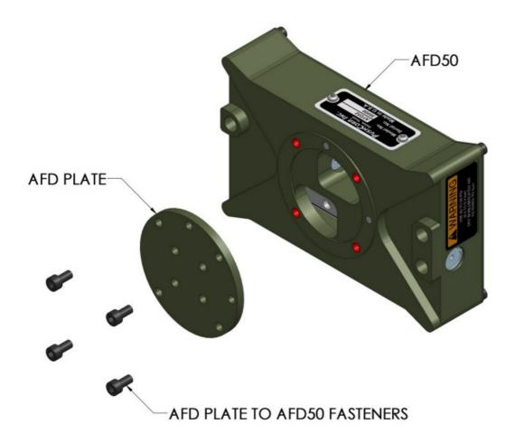
CAUTION: The Fastener Tightening Torque Specs chart in Section 6.0 should be used to determine proper fastener length and torque. This is to prevent pull out of the helicoil inserts
