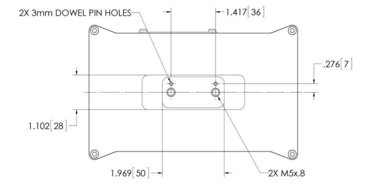
The Carriage has (2) two M5x0.8 mounting holes with a depth of 0.3 inch (7.5 mm) to provide secure attachment. The fasteners must thread in the proper distance to avoid helicoil pull-out at the recommended tightening torque (See Section 6.0). The mounting holes are spaced as shown Figure 2 above. The Carriage also incorporates (2)
