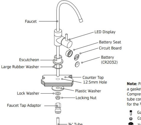
**Note:** Parts packet also contains a gasket, cone washer/olive & 1/4" Compression Nut, these are for a 1/4" tube connection and are not needed for the 3/8" installation.
