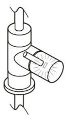
5. Red light flashes indicate your cartridges are due to be changed (usage has exceeded 3,000 minutes or 12 months).
