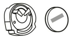
2. Install battery into the battery seat, positive side up.
