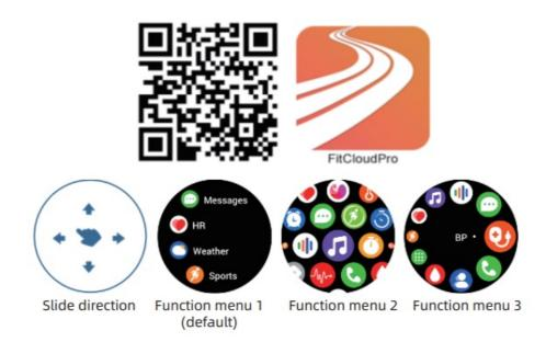
Touch all: Slide down to enter the status setting bar, slide up to view the notification, slide left to enter the main function interface, and slide right to enter the split-screen menu;
