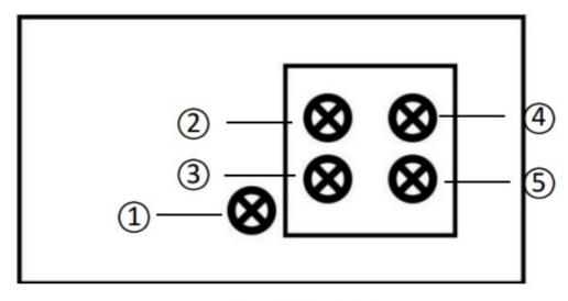
Screw 1: Ground wire Screws 2 & 3: Either of two live wires Screws 4 & 5: Not used
