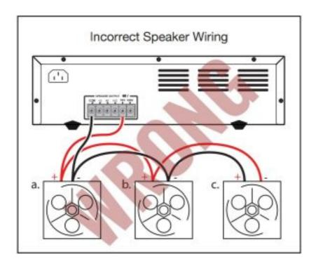
Be careful not to cross wires when installing your speakers. Wiring should always be negative to negative and positive to positive (Figure 2. shows speaker c. incorrectly wired).
