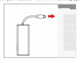
2. Use the USB C port for PD charging (Max up to 100W)
