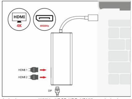
4. HDMI1 and DP port single plug support 4K60Hz, HDCP, HDR, HDMI2 port single plug support 4K30Hz, HDCP.
