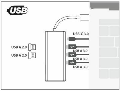
3. Connect USB peripherals to USB 3.0 ports on the hub three USBA 3.0 or one USB-C 3.0 data speed is up to 5Gops, and two USB 2.0 ports up to 480Mbps, please connect the wireless mice or keyboards through the USB 2.0 port.
