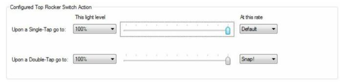
This setting determines what happens when you tab the rocker paddle to. Currently it is set to go to 100% at the default ramp rate. Using UPStart this can be changed to different settings:
