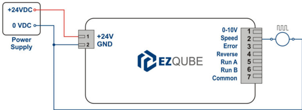
Figure 13 – SpeedOut PNP module wiring
