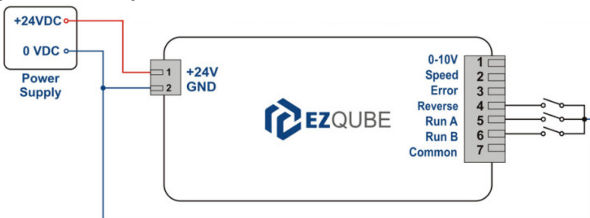
Figure 20 - NPN module wiring without Common connection
