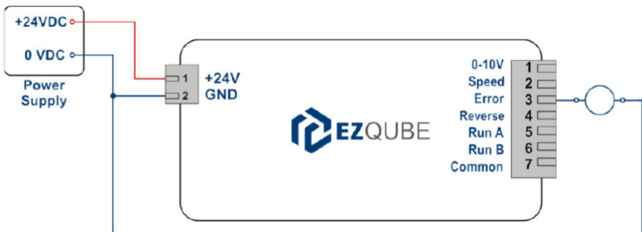
Figure 15 – ErrorOut PNP module wiring
