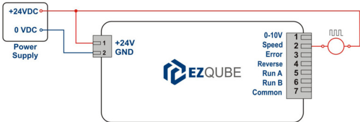
Figure 14 – SpeedOut NPN module wiring
