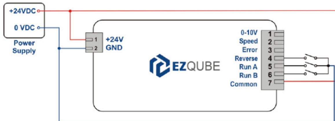
Figure 19 - NPN module wiring with Common connection
