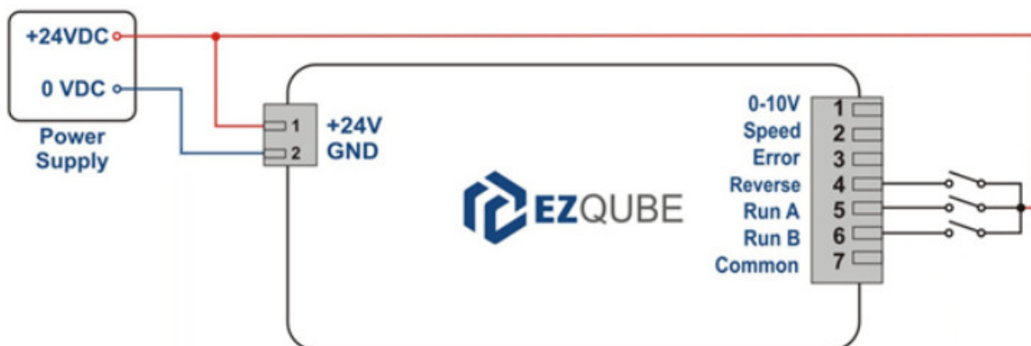
Figure 18 - PNP module wiring without Common connection
