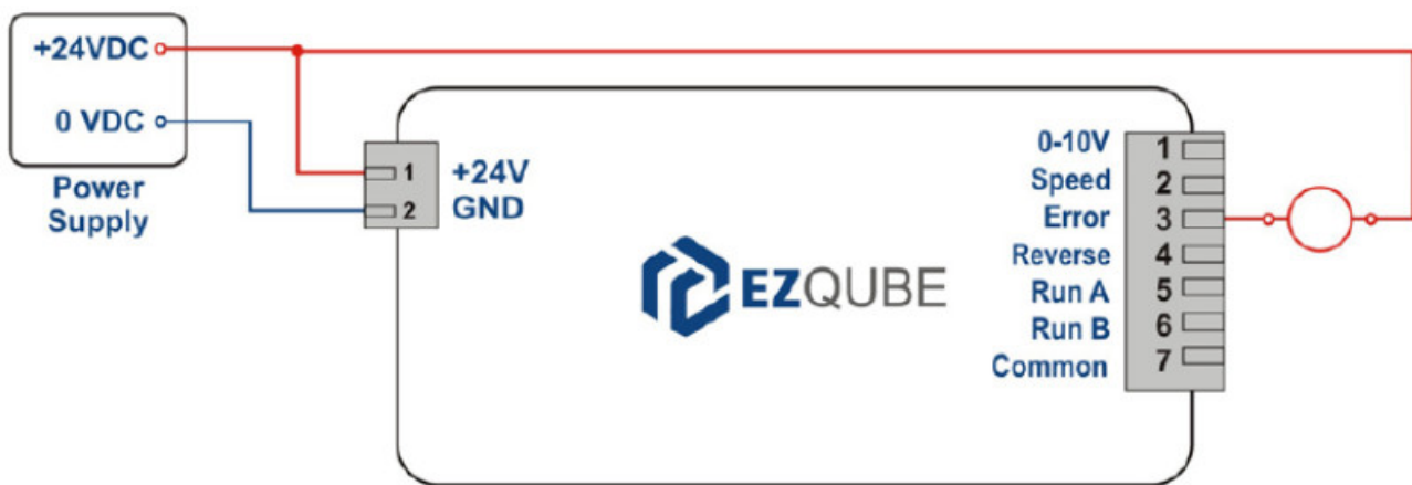
Figure 16 – ErrorOut NPN module wiring
