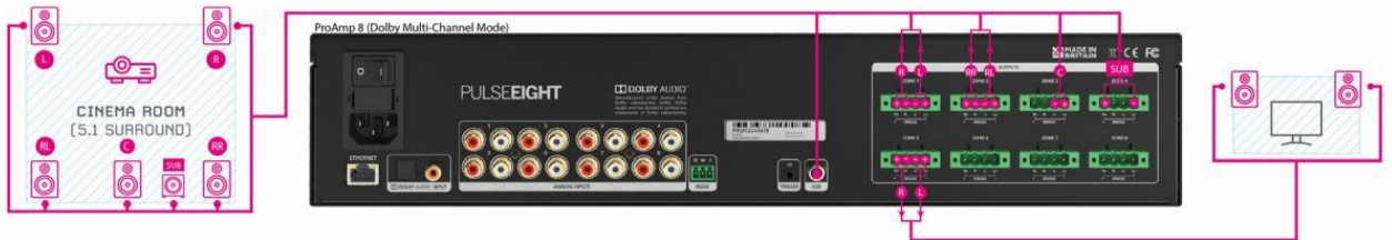
Figure 6: Connecting the audio output for 4 Zone Dolby Mode
