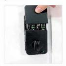
Remove the battery cover, install AAA1.5v batteries, and close the battery cover.
