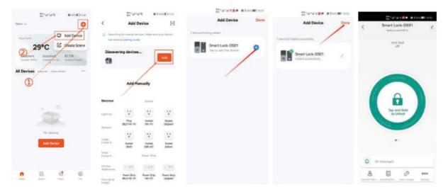
Start the distribution network process: If no fingerprint or password is entered, press any button or fingerprint to enter the distribution network mode, and the fingerprint or password has been entered, the machine automatically enters the distribution network mode;
