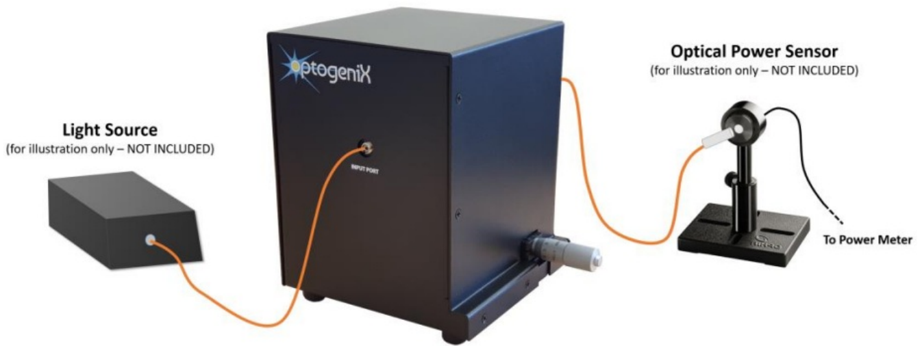
Figure 5 Setup for optical power calibration
