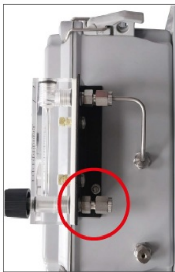
Figure 4 - Gas inlet (analyzer's right side elevation)
