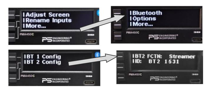
To pair the PMA450C PS Streamer with a compatible device, access the streamer menu from Radio-ICS →More →Streamer→ Config → Pair. Now, turn on the desired device and initiate the pairing on the device as well. This may take 60 seconds to complete.
