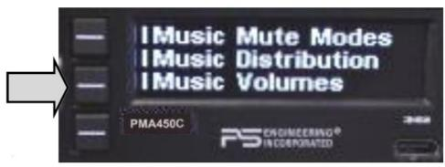
The PMA450C has two independent music inputs at the rear connector, and the ability to receive streaming music from either of two Bluetooth modules available in the PM4A50B, depending on how you have configured the audio panel.
