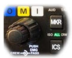
The outer, larger volume control knob controls intercom volume for the passengers. It has no effect on radio or music levels. When you turn the volume knobs, the green volume bar indicator will show the level of the changing intercom volume.
