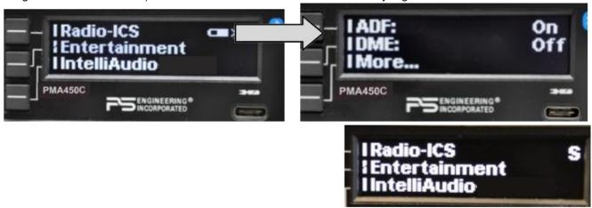
Additional navigation aid or other audio sources can be selected using the OLED menus. Press the top line select RADIO-ICS and select the desired audio source.
