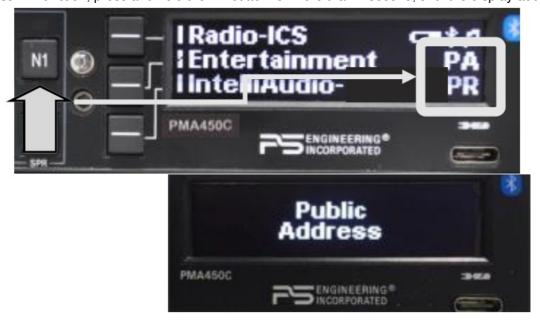
When the pilot is speaking on the PA through his microphone, all intercom except for the Pilot will be disabled for complete and uninterrupted announcements.
