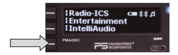
With IntelliAudio on, radio communication audio signals are digitally processed to "appear" in a different location to the pilot and copilot positions, specifically 10 o'clock for COM 1 and 2 o'clock for COM 2. This improve speech comprehension by locating it in a manner easily differentiated by the brain.
