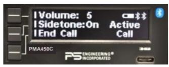
Some cell phones do provide sidetone, and when combined with audio panel sidetone audio distortion may occur. In PMA450C Telephone sidetone can be enabled or disabled on the Telephone menu which is active when a call is in progress.
