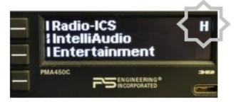
If you want to mute the audio over a marker station, pressing the MKR for one second causes the marker audio to mute for that beacon. The next beacon received will be heard. Marker Beacon sensitivity can be changed from Low to High sensitivity by pressing and holding the MKR button until "H" appears in the display, indicating High sensitivity is activated. Hold the MKR button again to set to Low sensitivity.
