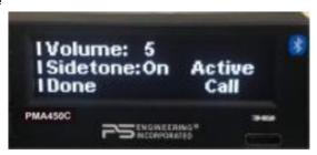
The PMA450C can accommodate a wired telephone input as well as a Bluetooth connection. However, only one can be active at a time. The Bluetooth icons are absent from the wired menu. The wired telephone screen menu is activated when audio is detected from the phone. Sidetone and telephone volume can be controlled from this menu. The telephone audio distribution is the same as Bluetooth, above. This menu will switch off 25 seconds after the incoming conversation ends, or press End Call.
