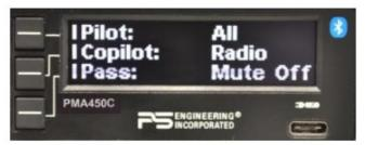
(**NOTE:** although phones can be connected to BT2, they can only act as streaming devices for music, not calls. Shown above, the pilot is connected to their phone (BT1) while the copilot is connected to the phone and to BT 2, which can send audio from Foreflight or music. BT2 can not be connected to a phone for telephone use, only entertainment.
