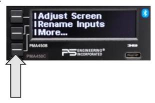
The first items are adjustments to the display, allowing the installer or user to tailor the display to suit the cockpit conditions. There are two functions: Display Brightness & Display Timeout. The display will vary in real time while adjustments are made. LED bar & numeric indication will vary.
