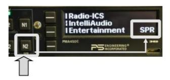
If you want to listen to your radios over the cockpit speaker, press and hold the N2 button (SPR is labeled under it) for 1 second or until SPR appears in the display.
