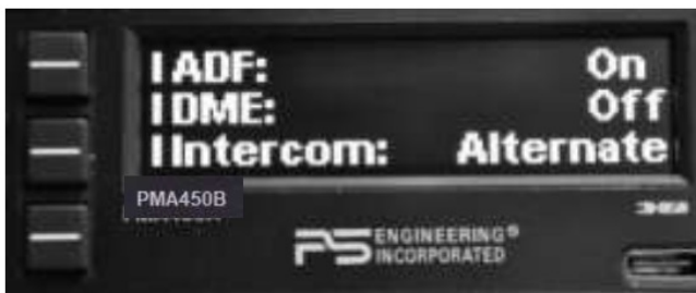
Alternate Intercom Mode enabled
