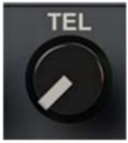
Once complete, you can press the TEL switch in to disconnectthe cell phone call.
