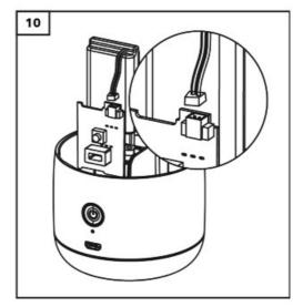
3. Remove the adhesive on the back of the battery, pull out the circuit board and the battery (fig. 9) and disconnect the battery from the circuit board (fig. 10). You can now safely remove the battery.
