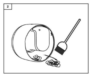
To open the lint compartment, twist the top counterclockwise (fig. 1) and remove it. You can then remove the lint inside (fig. 2). Make sure to empty the storage compartment before it is 80% full.
