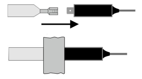
After connecting the antenna sensor, you can start placing the tape on the bumper by applying strong pressure in order to make it adhere well to its internal surface. After application, the excess part of the tape can be cut off.
