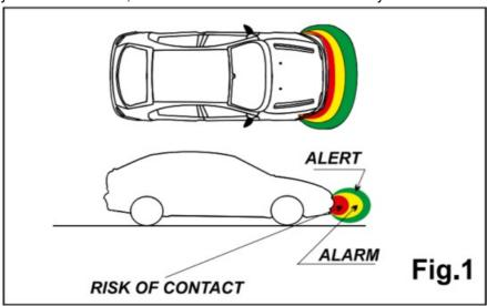
When approaching an obstacle the system activates the acoustic signal at a distance between the bumper and obstacle (measured in the central area of the bumper) of about 50/70 cm with 3 types of sounds:
