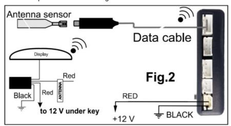
**NOTE:** Some vehicles are equipped with a metal crash protection bar insert facing the inside surface of the bumper. When this metal surface is too close to the inner surface of the bumper where you have placed the antenna sensor, the detection distance can be reduced.
