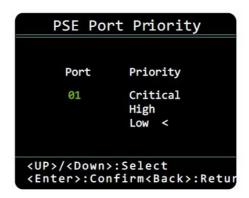
The PoE switch has a power bank (PB) measured in Watts (W). PD will require power from the power bank. This power will be marked as Total Power (TP). Once the TP is higher than the PB, the switch will automatically shut down ports in order not to overload and damage itself. PSE Port Priority allows the user to configure the priority of the ports – actually setting the order of which the ports will shut down.
