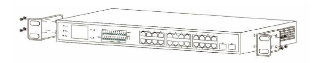
Step 2: Mounting the switch on the rack.
