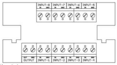
**OUTPUT:** 0-10VDC adder output
