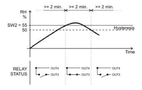
Cascade switching with two relays by VOC (NLII-iVOC+RH-R)
