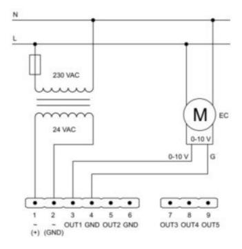
If you connect other devices to the same AC power source as the NL sensor, it is necessary to meet the GND wiring of all analog inputs and outputs, as well as power wires.
