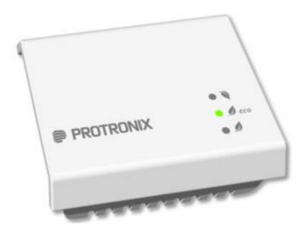
Room sensor NLII-iVOC is used to continuously monitor air quality inside buildings and then control ventilation (HVAC) systems according to current levels of air pollution. The sensor measures the concentration of gaseous organic substances in the air (VOC) and relative humidity (RH) of air. The sensor can be effectively used in offices, classrooms, restaurants, kitchens, fitness centers, commercial facilities, etc.
