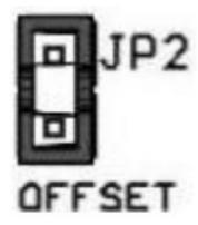
• Jumper not fitted = output 0-20mA.
