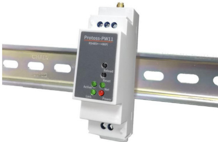
Figure 4. C45 Rail Installation
