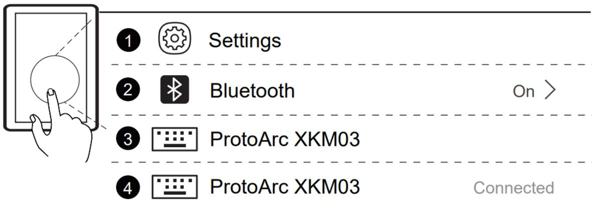
3. Turn on the Bluetooth settings on your device, search or select “ProtoArc XKM03” and start Bluetooth pairing until the connection is completed.
