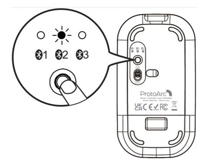
4. Turn on the Bluetooth settings on your device, search or select "XKM01 Mini" and start Bluetooth pairing until the connection is completed.
