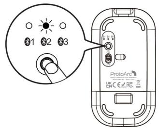
3. Long press the mode switch button for 3~5 seconds until the corresponding channel indicator flashes quickly, themouse enters Bluetooth paring mode.
