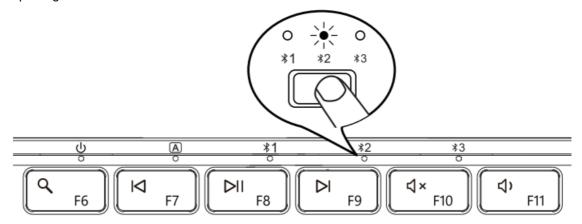
3. Turn on the Bluetooth settings on your device, search or select "ProtoArc XK01 Plus "and start Bluetooth pairing until the connection is completed.
