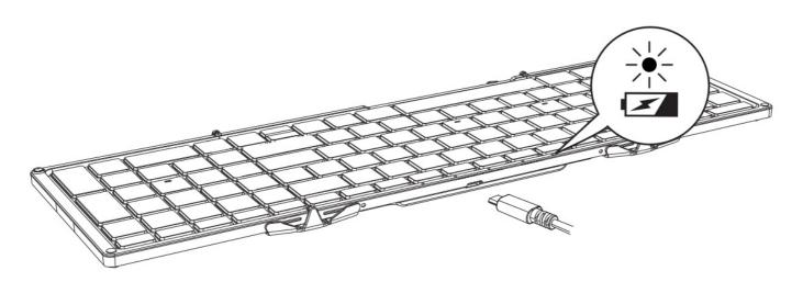
When the battery is too low, the low battery indicator will turn red and flash quickly. Please connect to the power supply to charge in time to ensure that the keyboard has sufficient power to meet normal work. If the battery of the keyboard is too low, there will be delays freezes, and other problems in typing, which affect normal use. The power indicator turns red while charging, then turns off after fully charging.
