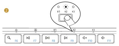
3. Turn on the Bluetooth settings on your device, search or select "ProTour XK01" and start Bluetooth pairing until the connection is completed.
