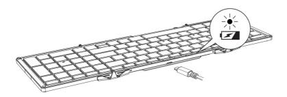
When the battery is too low, the low battery indicator will turn red and flash quickly. Please connect to the power supply to charge in time to ensure that the keyboard has sufficient power to meet normal work. If the battery of the keyboard is too low, there will be delays and freezes and other problems in typing, which affect normal use. Power indicator turns red while charging, then turn off after fully charged.
