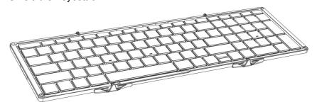
2. Single press to choose any Bluetooth connection, the blue indicator light flashes once to enter Bluetooth mode. Then long press for 3-65, when the blue indicator light flashing quickly, it enters Bluetooth pairing mode.
