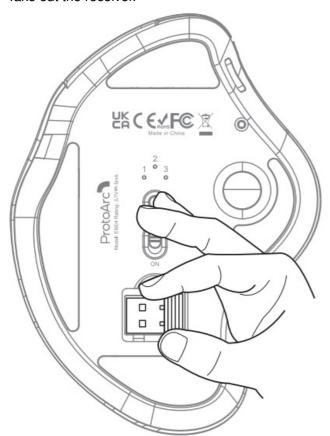
3. Press the channel switch button until the channel 1 flashes a white light, and the mouse enters 2.4G wireless mode.
