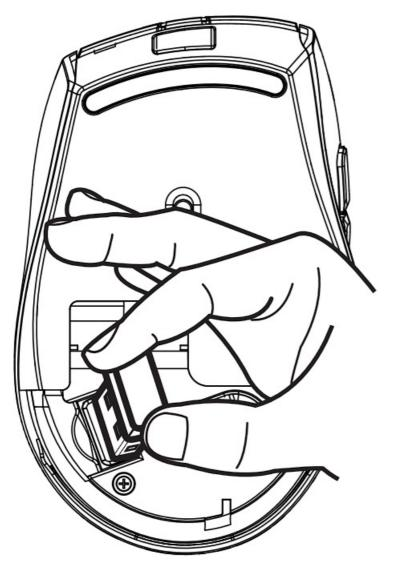
3. Plug receiver into the USB port.
