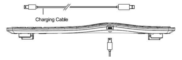
When the battery is low, the white indicator light on the button of the channel in use will start to flash until the device shuts down. Please charge the keyboard as soon as possible to ensure it has sufficient power for stable connection. If the battery is
