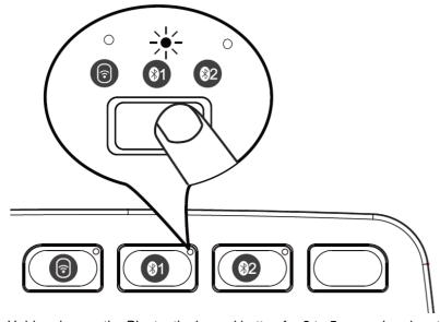
3. Hold and press the Bluetooth channel button for 3 to 5 seconds, when the white indicator light starts flashing quickly, it
