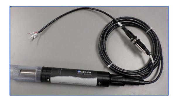
If you wish to retrofit a Proteus with the MIB option, please contact us. If you wish to build your own MODBUS or SDI-12 converter cable, or convert your Underwater Cable into a converter cable, use the wiring diagrams in Appendices One and Two.
