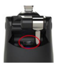
Note: Tighten until flush plus 1/2 turn (equivalent to 80oz-in torque).
