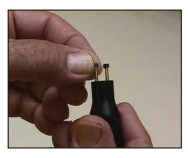
2. Conductive rubber boots are used to reduce contact resistance between the electrodes and material under test. Measurements made with bootsinstalled are typically lower than those obtained without boots.
