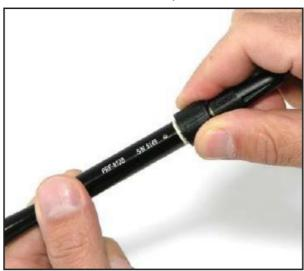
2. Connect measurement cable to Dual Banana BNC Converter (Figure 3).
