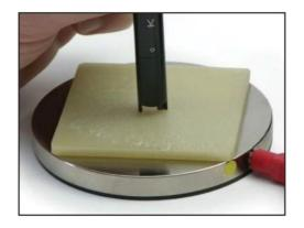
Figure 7 shows the classic setup for measurement of a material's resistance in accordance with ANSI/ ESD STM11.12 Volume Resistance. It also provides an indication of the material's probable resistance to ground (Rtg) when in use and while in contact with a grounded conductive surface. Note that this measurement is not an actual Rtg measurement. It is simply an indication that the material or DUT may be Groundable, depending on its measured resistance characteristics.
