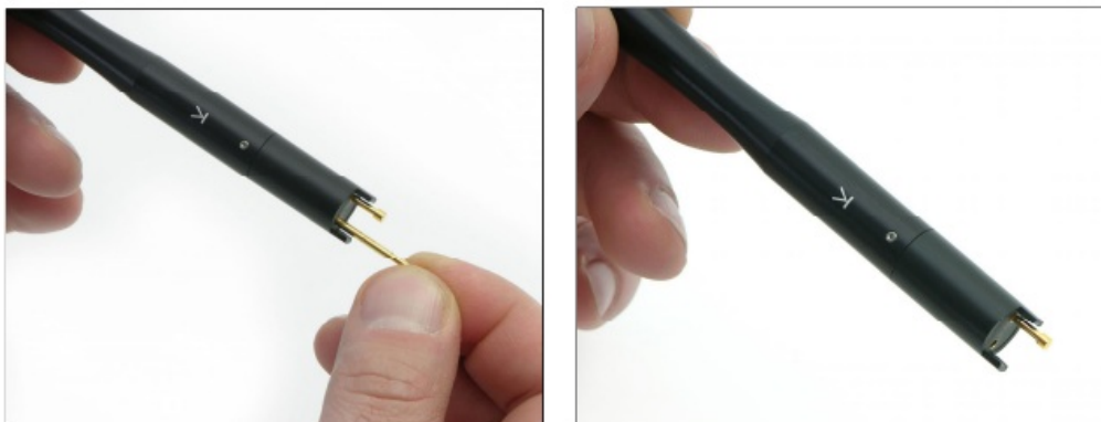
Figure 11. Removing the inactive pin helps identify point of actual measurement by the active pin.
