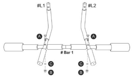
2. Connect bar #L1 and bar #L2 to #Bar1 using screws A, spring washers C and nuts B. Do not tighten up any nuts fully before #Bar2 is connected to bar #L1 and bar #L2.
