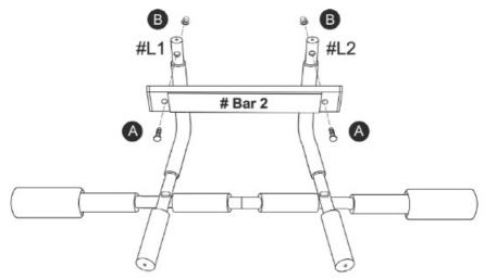
3. Connect #Bar2 to bars #L1 and #L2 using screws A. Tighten up all nuts so that the whole unit is straight.
