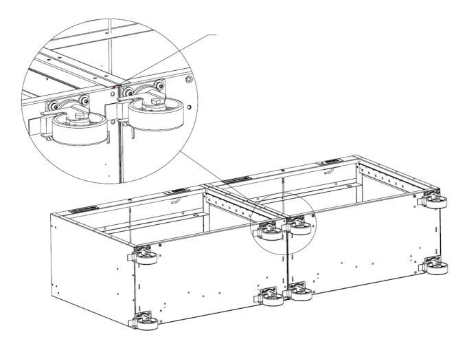
In the case of attaching two main CORE together. To avoid interference of two casters at the connecting sides. In one of the cabienet install casters at provided offset holes.
