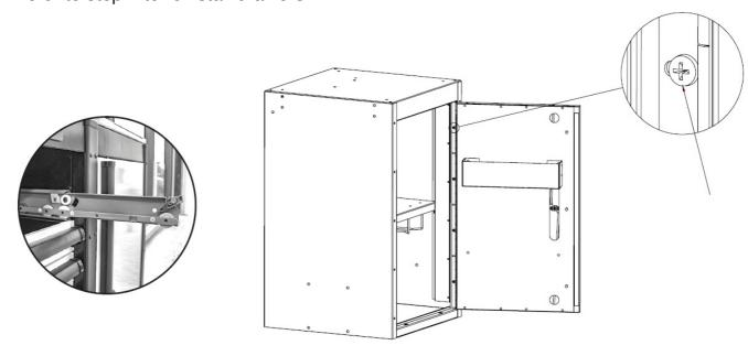
Open all the screws to be able to remove the door.
