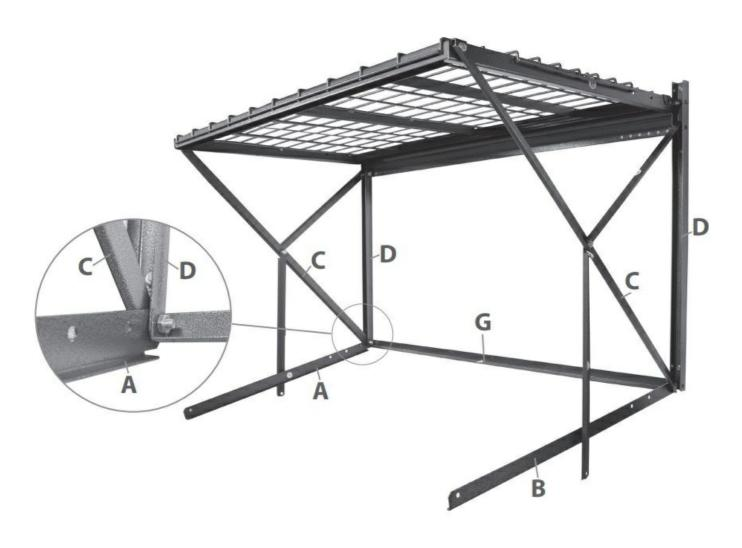
**Step 3**Connect one of your crossmembers F to I & A. (front) Then, connect the same F bar to J & B. Connect rear crossmember F by overlapping it with A & B parts. Use last hole of A & B.
