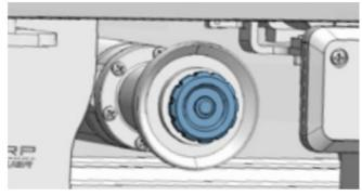
4. Replace with a new grinding wheel, set in place. Do not push on with force, just place on the spindle and turn wheel lock clockwise while holding grinding wheel until snug.
