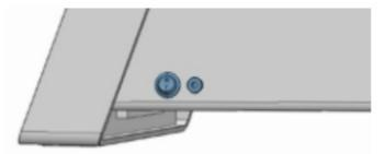
3. Unscrew the grinding wheel lock (counterclockwise) while holding the grinding wheel in place. Wheel is snug, pull off carefully without excessive force while rocking the grinding wheel off the spindle.
