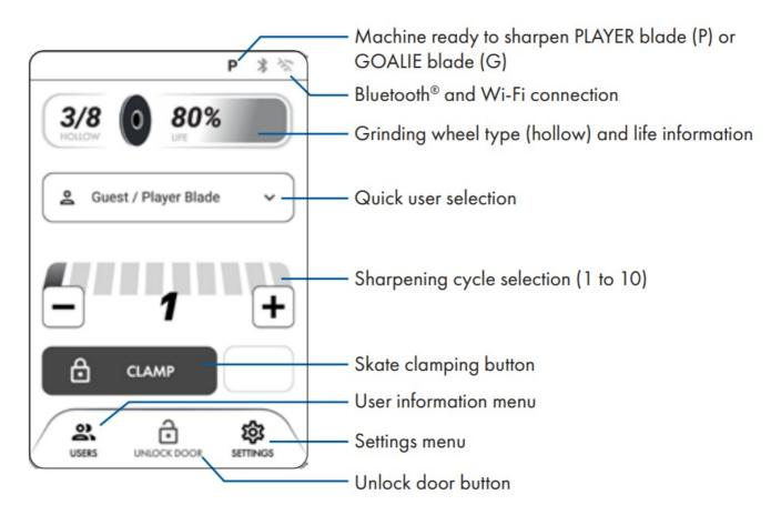
After pressing "CLAMP", the buttons will change to "START". To unclamp the skate, press the gray unlock icon.
