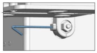
2. Place the adjustment tool into the hexagonal adjustment nut located inside the machine.
